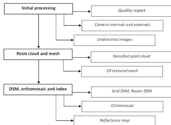
**Figure 5.** Technological scheme of creating an orthomosaic in Pix4D.
