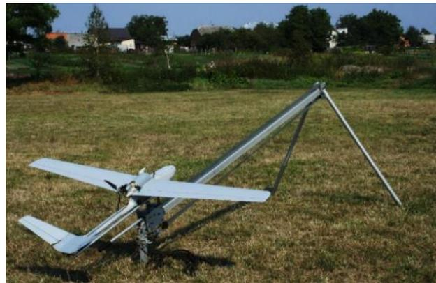
Figure 2. General view of the Arrow UAV before launch
