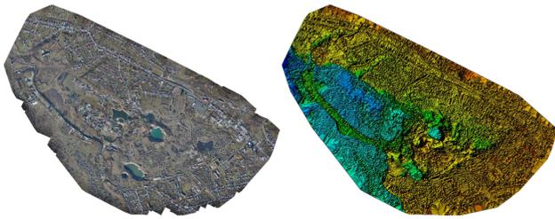
Figure 6. Orthomosaic and DTM created in the Pix4D software package.
