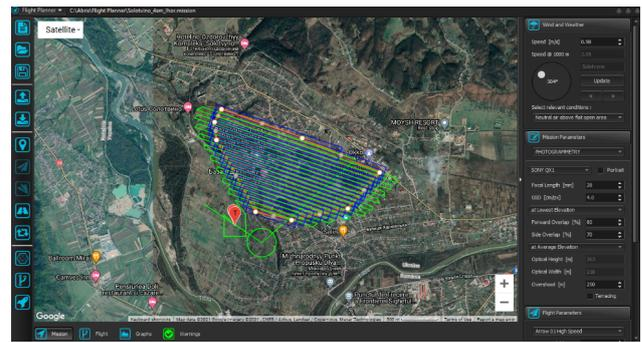
**Figure 3.** Designed flight routes.
