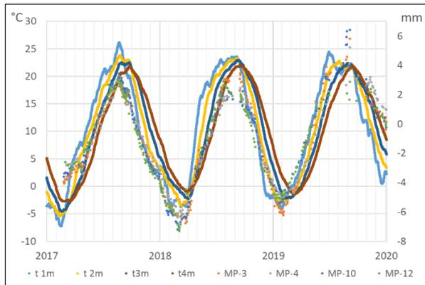
**Figure 12.** Average temperature values (1, 2, 3, 4 months) and horizontal displacements of points MP-3, MP-4, MP-10 and MP-14
