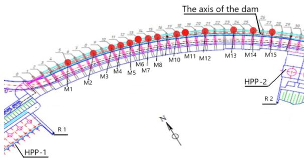
Figure 4. Diagram of the location of GNSS control points MP1–MP15 on the dam of the Dnieper Hydroelectric Station
