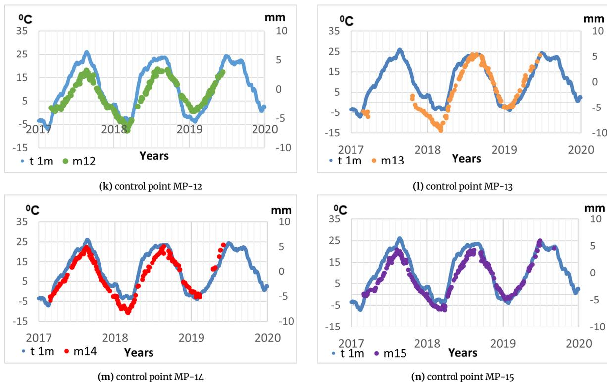
Figure 13. Average values of temperature (1 month) and horizontal displacements of GNSS control points
