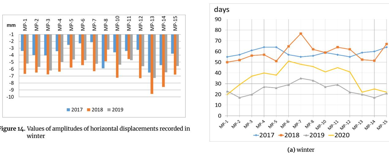
Figure 14. Values of amplitudes of horizontal displacements recorded in winter
