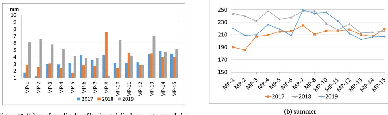
Figure 15. Values of amplitudes of horizontal displacements recorded in summer
