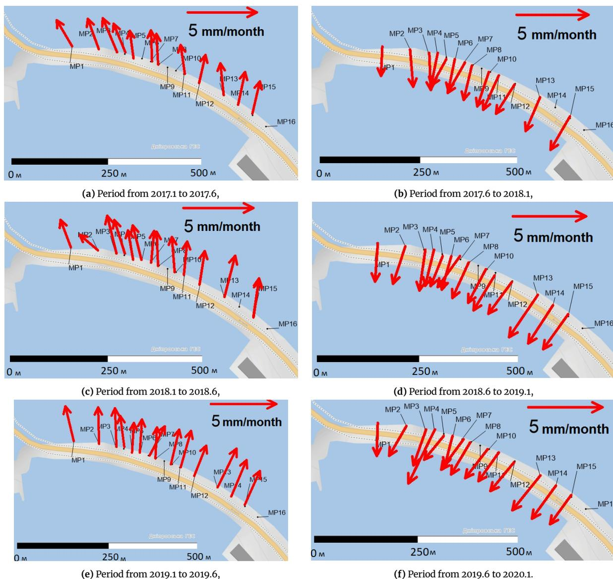
**Figure 6.** Distribution of velocity vectors of control points horizontal displacements of the Dnieper Hydroelectric Station dam from 2017.1 to 2020.1
