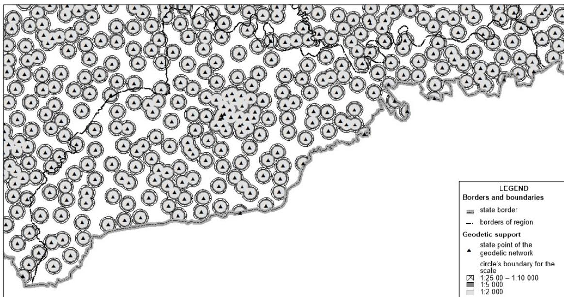
Figure 1. Schematic representation of geodetic support by the method of construction of buffer zones (fragment)
