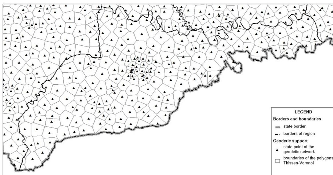
Figure 3. Schematic representation of geodetic support by the Thissen-Voronoi method (fragment)
