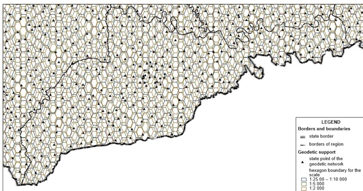
Figure 2. Schematic representation of geodetic support by the method of construction of a hexagonal grid (fragment)
