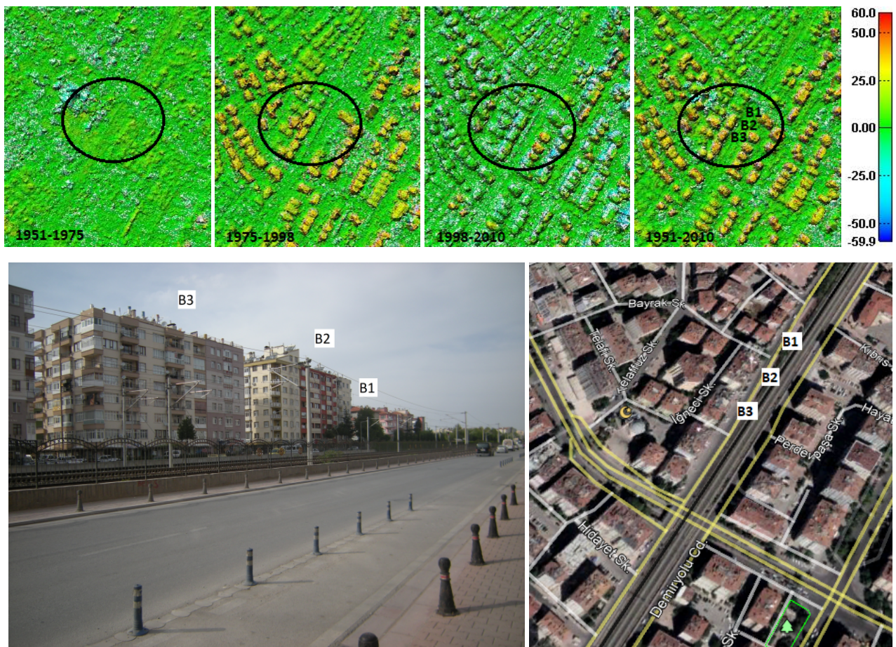
Figure 10. The visualization of changes in comparison of time series point clouds (B1 location: 37^{\circ}53'09.15'' N latitude, 32^{\circ}29'08.37'' E longitude) (Legend unit: meter)
