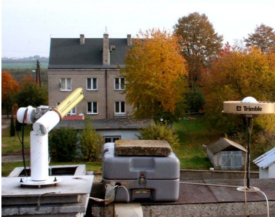
Fig. 2. CIMEL-318 and GPS antenna at Belsk
