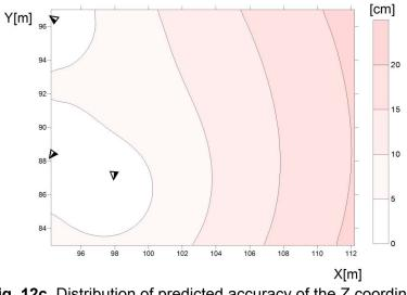
Fig. 12c. Distribution of predicted accuracy of the Z coordinate (3 sensor – configuration of the practical test)
