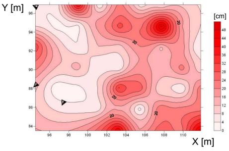
**Fig. 11c.** Graphical presentation of differences dz between the coordinates obtained from the Ubisense system and the TCRP 1201+ for a configuration of 3 sensor stations
