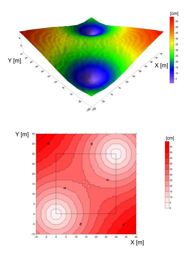
Fig. 10c. Distribution of predicted accuracy of the Z coordinate (2 sensor stations mutually turned to each other)
