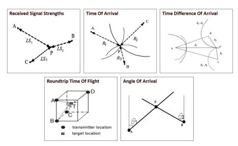
Fig. 2. 3D positioning principles (Ubisense)
