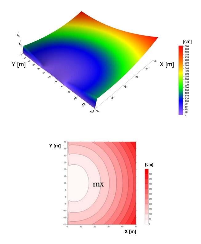
Fig. 8a. Distribution of predicted accuracy of the X coordinate (2 sensor stations turned in the same direction)
