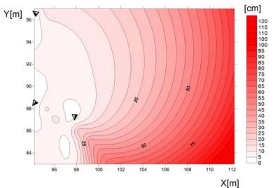
**Fig. 12a.** Distribution of predicted accuracy of the X coordinate (3 sensor – configuration of the practical test)
