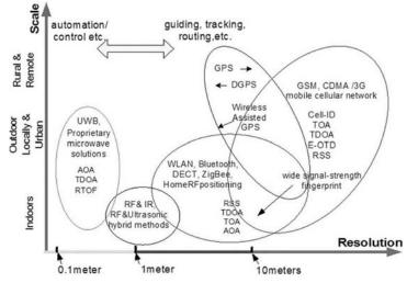
Fig. 1. Positioning systems overview (Liu et al., 2007)
