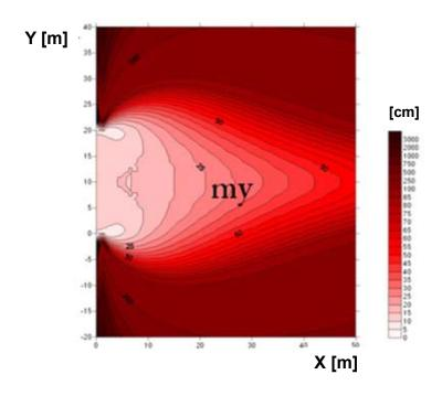
Fig. 8b. Distribution of predicted accuracy of the Y coordinate (2 sensor stations turned in the same direction)
