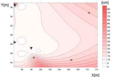
Fig. 12b. Distribution of predicted accuracy of the Y coordinate (3 sensor – configuration of the practical test)
