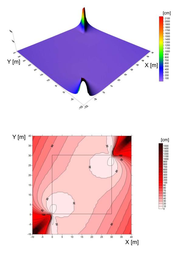
Fig. 10a. Distribution of predicted accuracy of the X coordinate (2 sensor stations mutually turned to each other)
