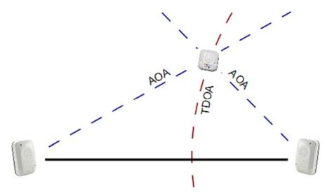
Fig. 6. The object location as an intersection of lines and surfaces
