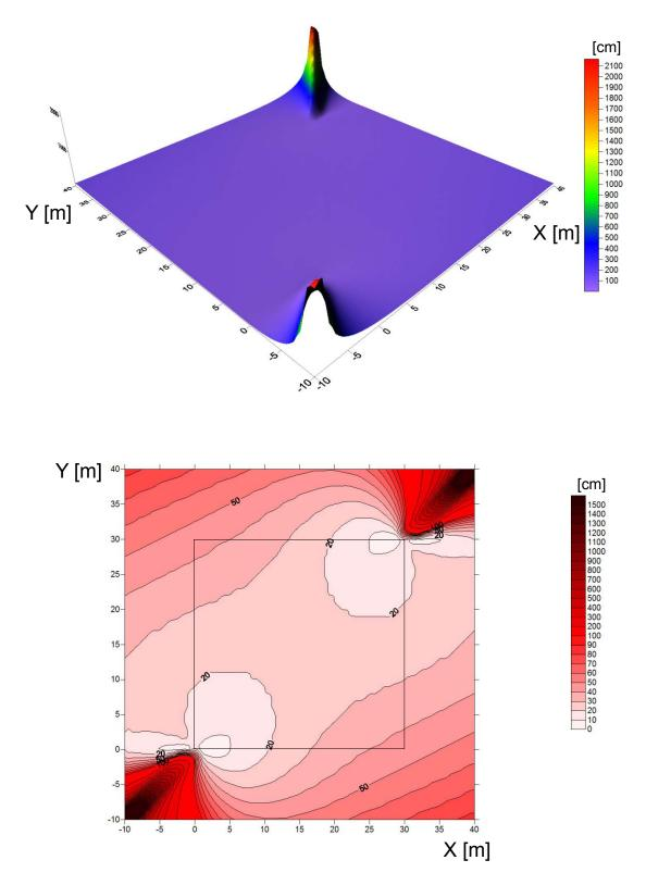
Fig. 10b. Distribution of predicted accuracy of the Y coordinate (2 sensor stations mutually turned to each other)
