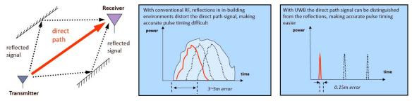
Fig. 3. Noise elimination of signal multipath
