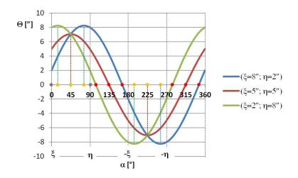
Fig. 2. Quasigeoid to ellipsoid slope in characteristic directions
