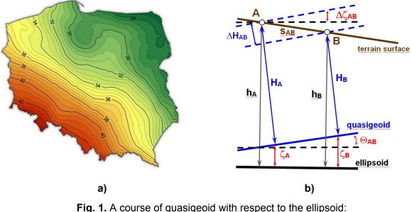
Fig. 1. A course of quasigeoid with respect to the ellipsoid:
