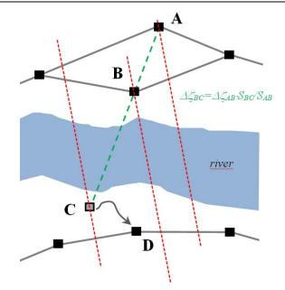
Fig. 4. Outline of the use of information on the course of quasigeoid in leveling through field obstacles in method II
