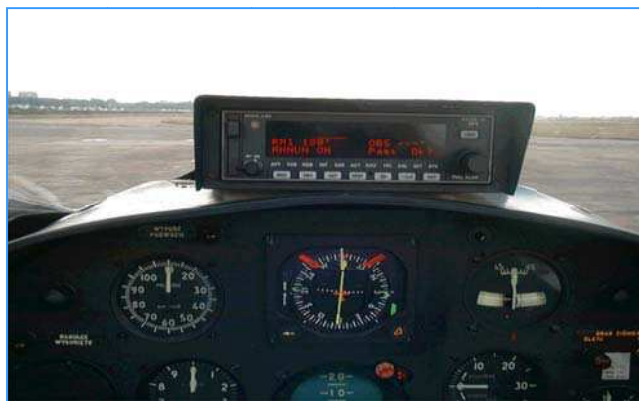
Fig. 2. An on-board GPS receiver KLN 89 mounted in Polish aircraft TS-11 "Iskra"
