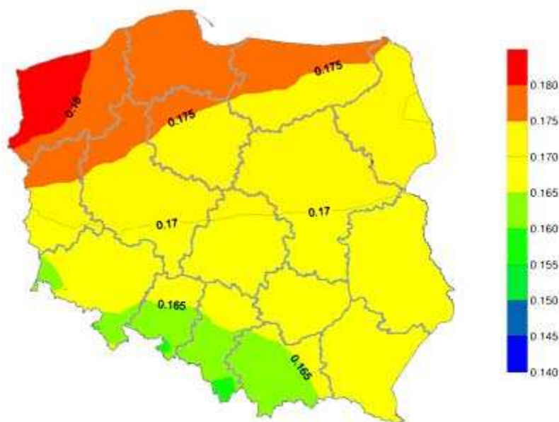
Fig. 8. Height differences between reference frames KRON2006 and PL-EVRF2007-NH
