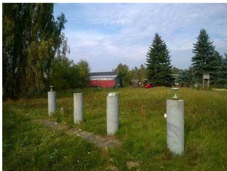
**Fig. 12.** Points of GNSS field calibration test baseline at WUT Józefosław Observatory
