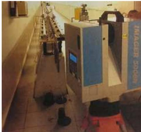
**Fig. 23.** Position of scanner relative to interferometric comparator
