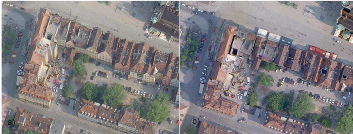
Fig. 2. Examples of: orthophotomap (a), true-orthophotomap (b)
