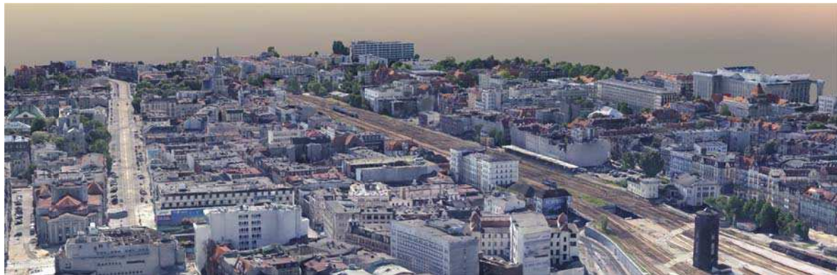
Fig. 3. Example of Katowice 3D model based on oblique aerial images
