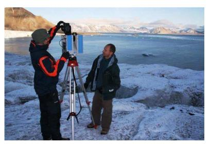
Fig. 14. First test of Z+F Imager 5006 scanner with integrated digital camera on Hans Glacier in 2007. Artur Adamek on the right (W. Krawiec).
