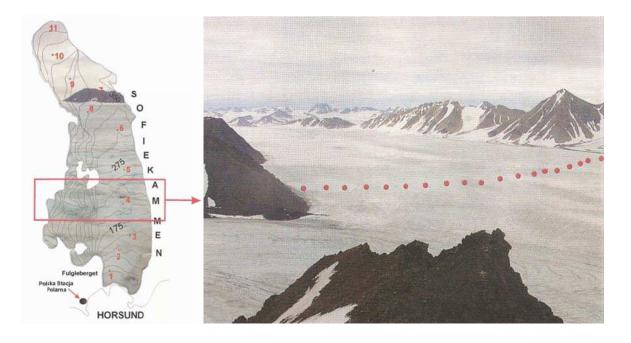
Fig. 11. Ablation pole placement on Hans Glacier in longitudinal and transverse profiles (Węzka et al., 2006)
