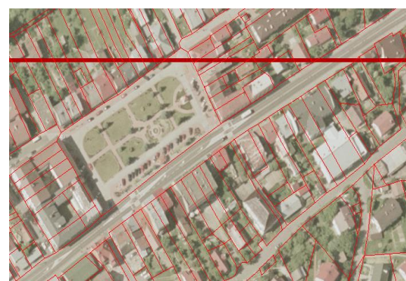
Fig. 6. Comparison of EGiB vector map after modernization with an orthophotomap in built-up areas (own research based on PODGiK data)
