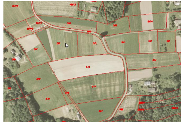
Fig. 8. Comparison of EGiB vector map after the modernization with an orthophotomap in the poorly invested area (own research based on PODGiK data)
