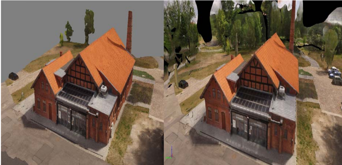
Fig. 4. Image (Texture) generated by the tested software: (on the left – Agisoft Photo Scan Professional Edition, on the right – Pix4D Pro mapper)
