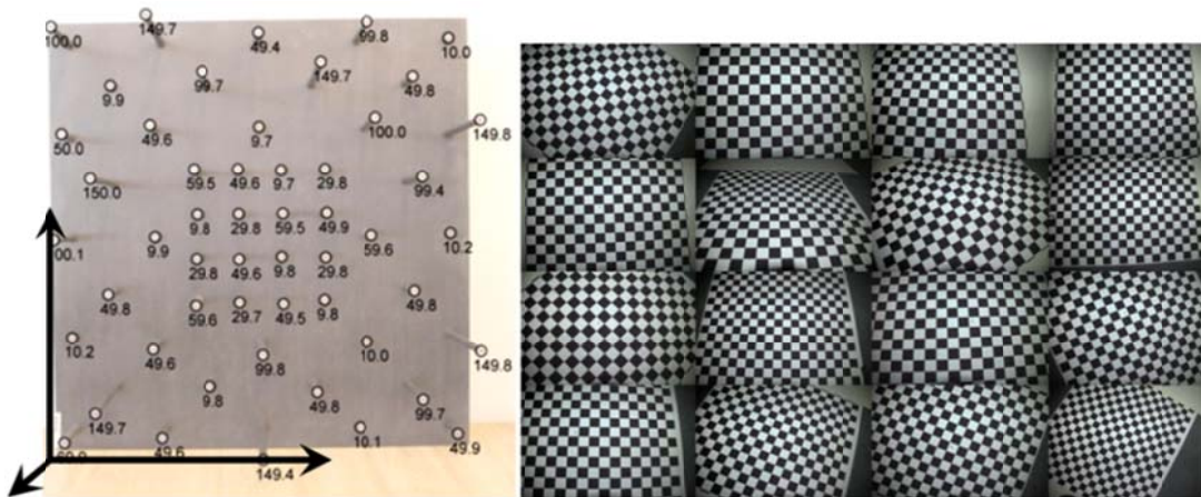
Fig. 1. Calibration tests 3D and 2D for very large close range photographs (Bujakiewicz et al., 2006b)
