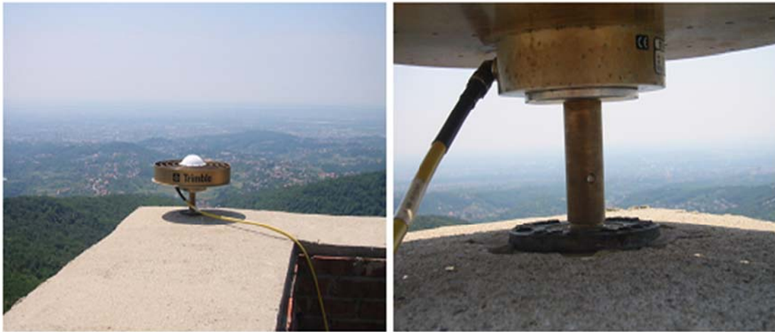
Fig. 6. Stabilisation of GPS antenna above the point (Đapo, 2009)
