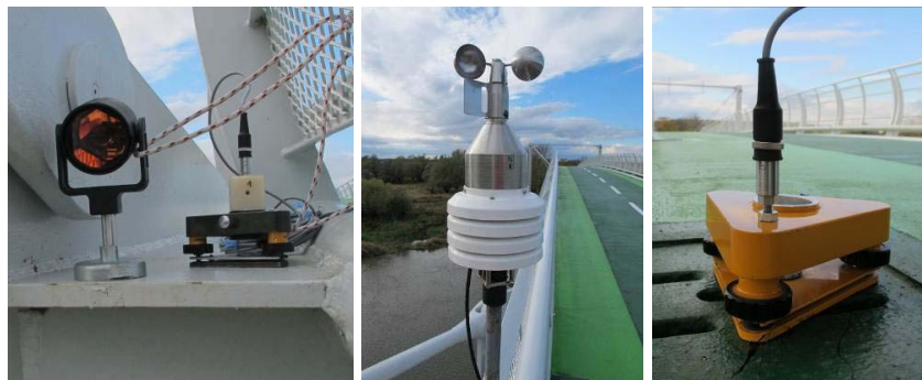
Fig. 3. Stabilization of the sensors on the bridge deck
