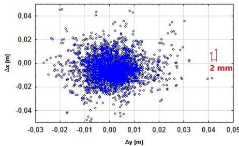
**Figure 6.** Summary of the scatter (x, y) of all measurements
