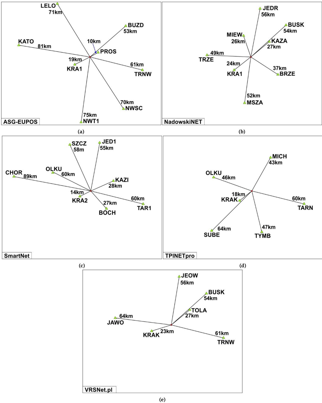
Figure 4. CORS network geometry for the test measurement site: (a) ASG-EUPOS, (b) NadowskiNET, (c) SmartNet, (d) TPINETpro, (e) VRSNet.pl
