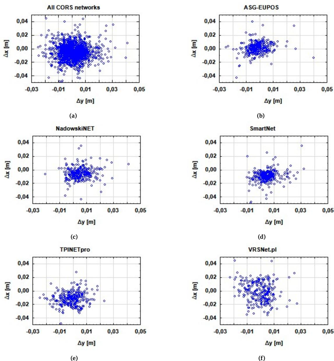
Figure 5. Scatter of (x, y) measurement positions: (a) All CORS networks, (b) ASG-EUPOS, (c) NadowskiNET, (d) SmartNet, (e) TPINETpro, (f) VRSNet.pl
