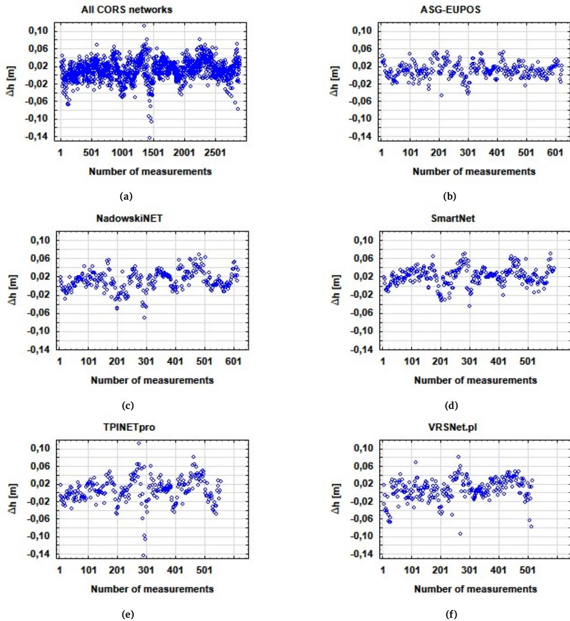
Figure 7. Scatter of heights on the timeline (described by the number of measurements): (a) All CORS networks, (b) ASG-EUPOS, (c) NadowskiNET, (d) SmartNet, (e) TPINETpro, (f) VRSNet.pl
