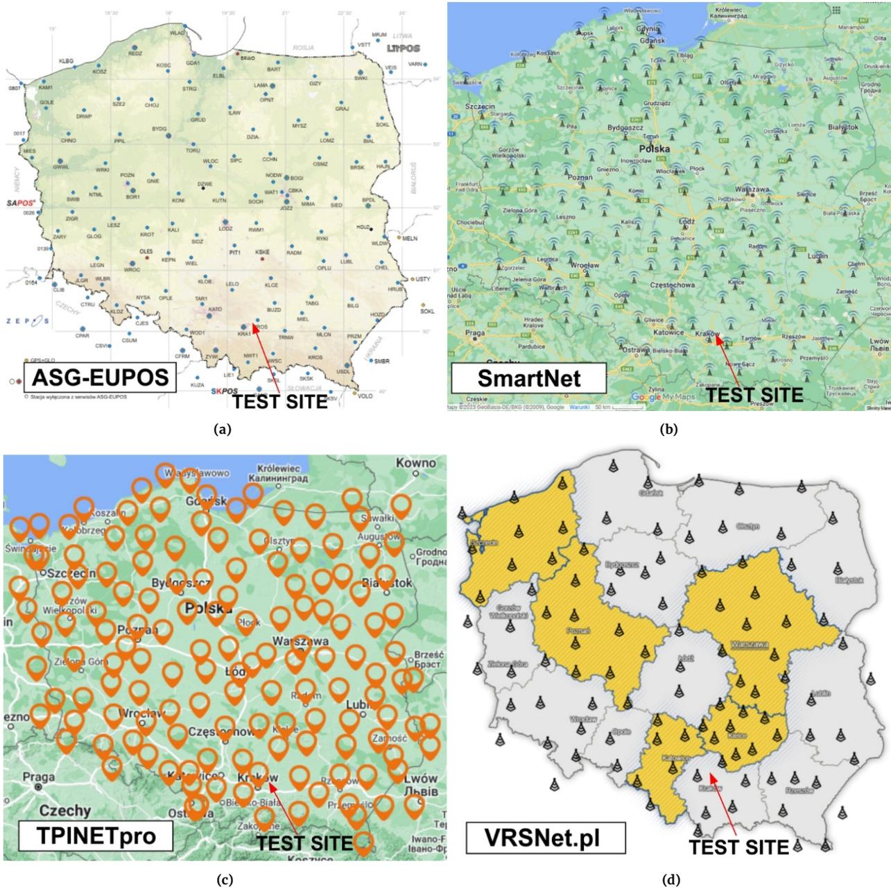
Figure 1. Location of reference stations of nationwide CORS network in Poland: (a) [www.aseupos.pl](http://www.aseupos.pl), (b) <https://pl.nrtk.eu/>, (c) <https://tpinet.pl/>, (d) <http://vrsnet.pl/>
