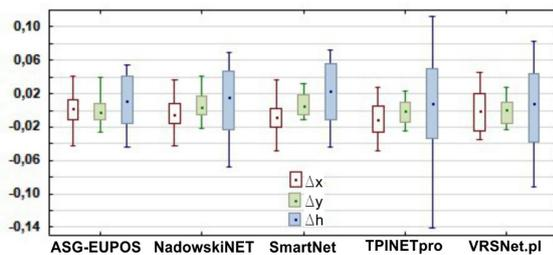
**Figure 8.** Whiskers box in [m]: median, bar: 90% of observations, whiskers: min-max
