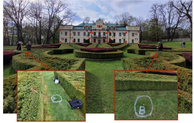
Figure 7. Total station measurement from two stands to the tie points located on the front facade of the Mioszowski Palace, reference points on objects surrounding the palace, and the control points mounted along the main crack
