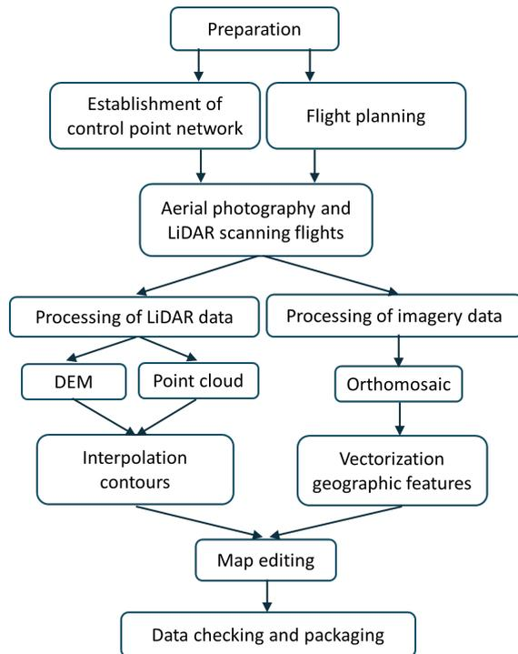
**Figure 3.** Topographic surveying process in the Win 3 Wind Power Plant project area using UAV LiDAR
