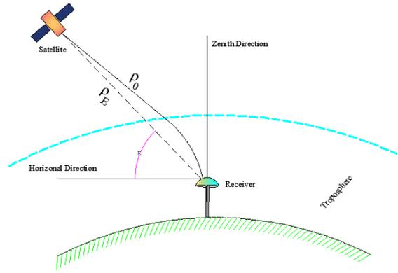
**Figure 1.** Tropospheric delay as the difference between the optical path of the electromagnetic wave and the geometric path
