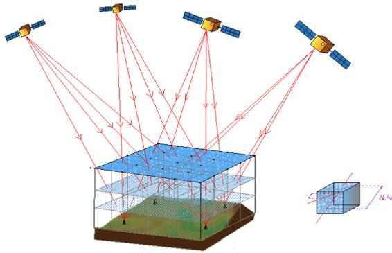
Figure 2. GNSS tomography by discretization
