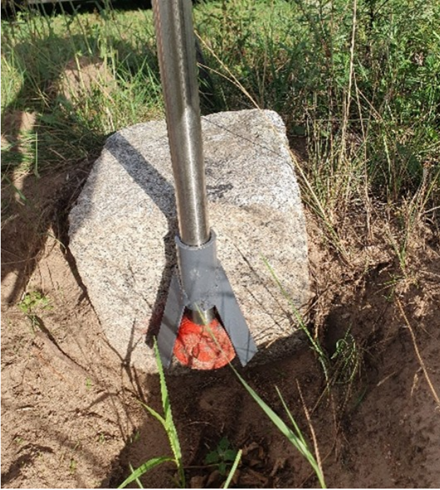
Figure 7. Accurate centering of the instrument for precise forced centering of a GNSS antenna on a benchmark of about 63 mm in diameter with horizontal axis orientation, using a triangular head
