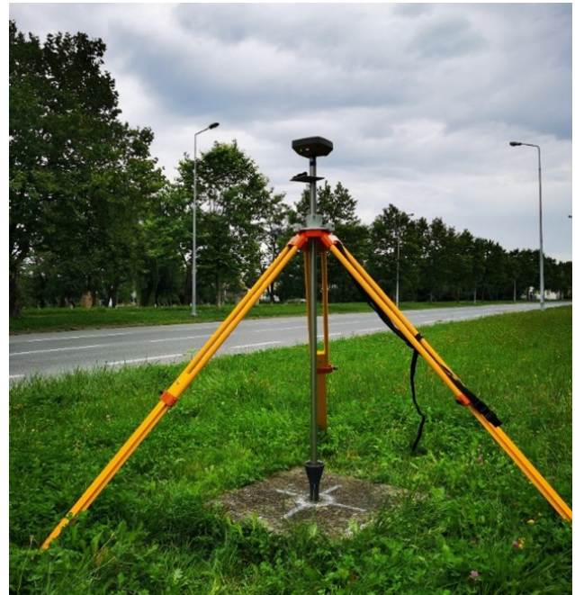
Figure 6. Static GNSS measurement on a vertical network point using an instrument for precise forced centering of the GNSS antenna
