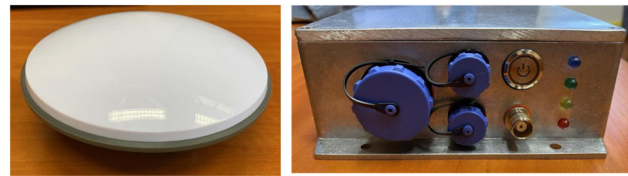
Figure 4: Equipment used in the experimental measurement: GNSS antenna and low-cost GNSS receiver
